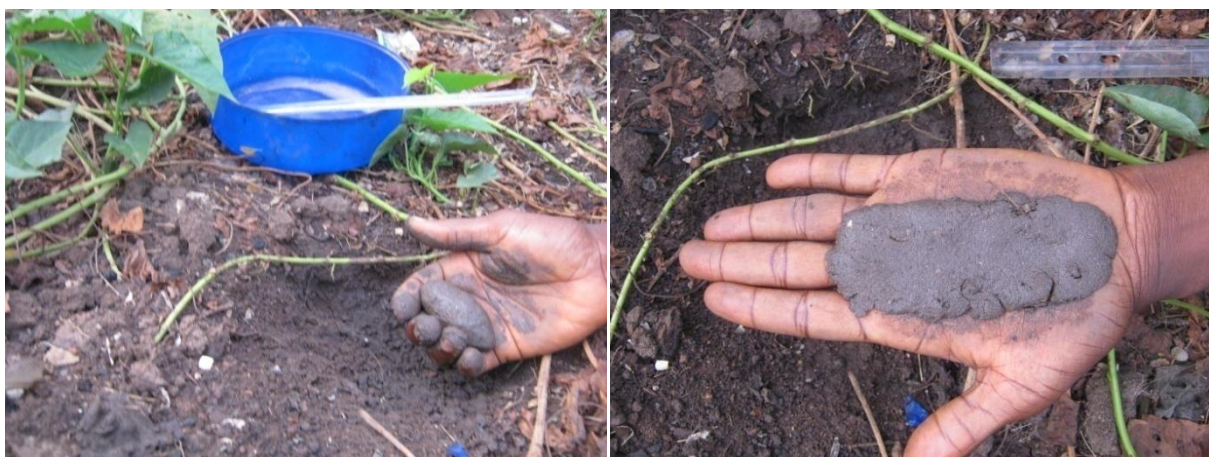
Fig. 4: Field soil textural analysis (a) threading of soil into bolus (b) bolus pressed out to form a ribbon
